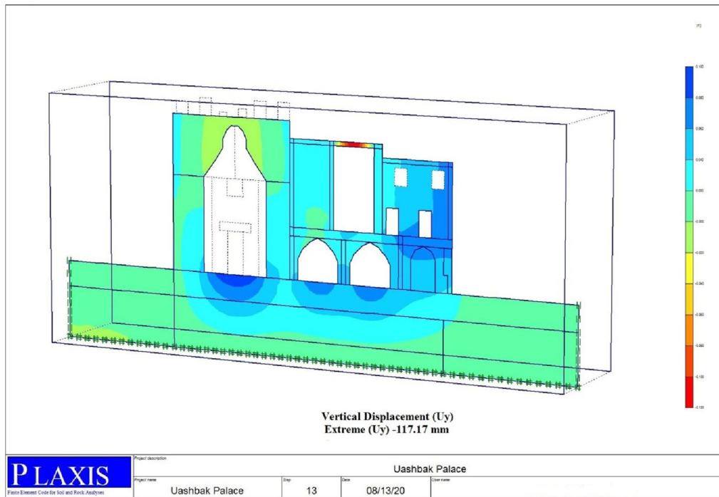
Fig. 18 Details of the induced vertical displacement of the super structure and bearing soil of Qasr Yashbak due to the primary and secondary consolidation settlement
