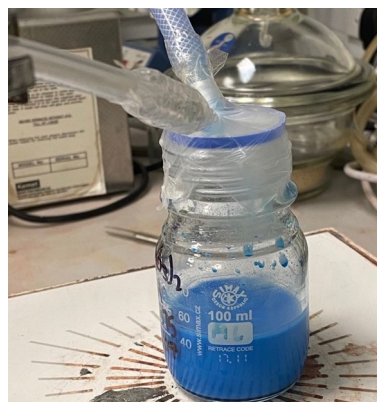
Fig. 2 CO 2 atmosphere reaction vessel setup; inlet and outlet CO 2 lines are secured in vessel
