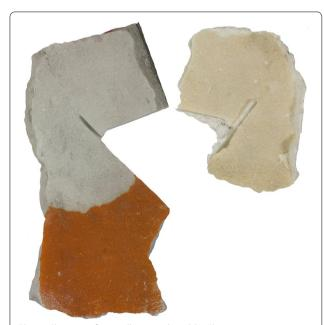
**Fig. 5** Cleaning of naturally stained marble. Cleaning experiment of naturally stained *Greenlandic* marble showing a cleaned and an uncleaned area. The piece at the *right* shows the poultice after removal. Height of sample: c. 16 cm. Cleaning solution: 0.1 M cys + 0.1 M SD
