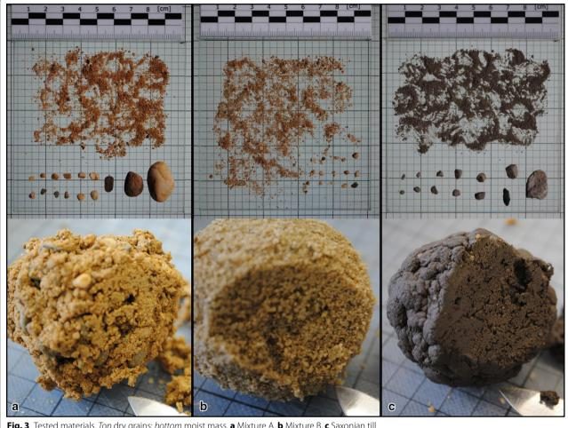
Fig. 3 Tested materials. Top dry grains; bottom moist mass. a Mixture A, b Mixture B, c Saxonian till
