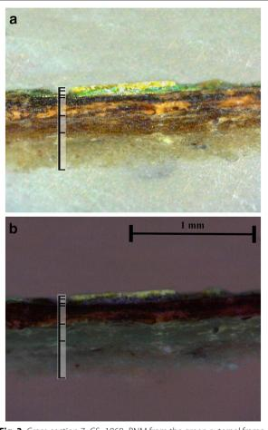
Fig. 3 Cross-section 7\_CS\_1869\_BNM from the green external frame of the painted decoration. From the top: yellow varnish, green colour, gold leaf, leather, adhesive, pasteboard. Binding, left board. Images © Biblioteca Nazionale Marciana, Venice. **a** VIS light, ×200. **b** UV light, ×200
