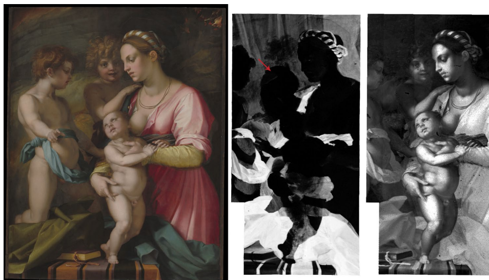
Fig. 3 (Left) color image of Andrea del Sarto's Charity , Samuel H. Kress collection, National Gallery of Art, Washington D.C. Photo Mr. G. Williams, (middle) Copper (Cu K \alpha ) map, (right) inverted natural log of Iron K \alpha map. Dark areas denote where iron was found. Note in the Cu K \alpha map the head of a man can be seen in reserve (red arrow), in the area of the chest and chin of the boy in the middle of the painting
