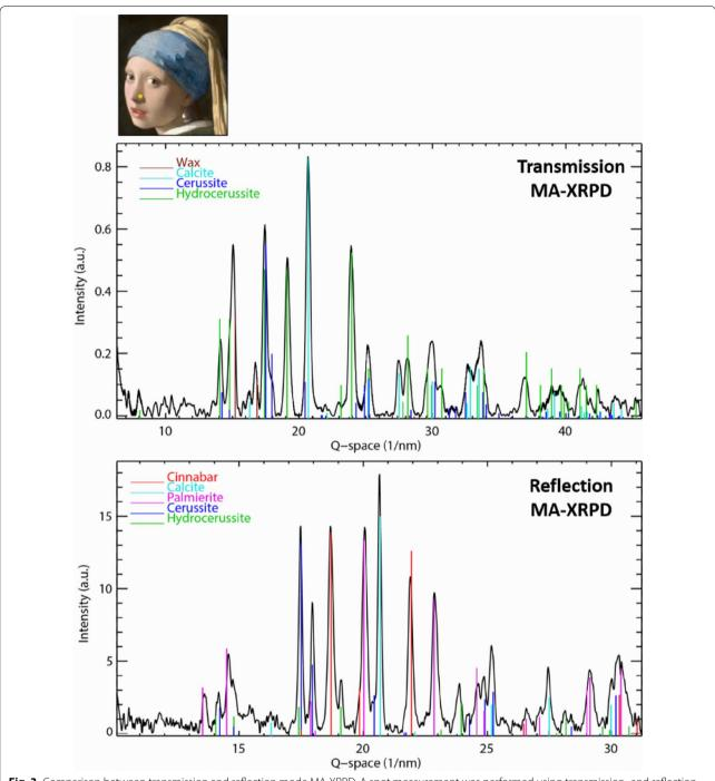
**Fig. 3** Comparison between transmission and reflection mode MA-XRPD. A spot measurement was performed using transmission- and reflection mode MA-XRPD on the nose of the Girl. The yellow dot indicates the position where the measurement was performed
