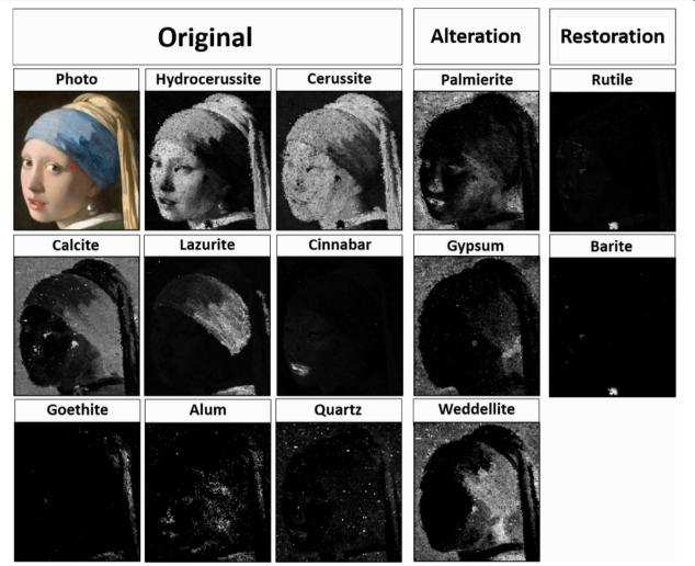
Fig. 2 Results obtained with MA-rXRPD. Distribution images obtained with MA-rXRPD showing the scaling parameter for every pixel. Higher scaling parameters are represented by a brighter colour. The position where the paint fragment for μ-XRPD analysis was taken is marked with a red dot
