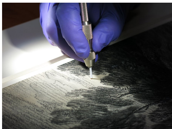
Fig. 2 Sampling of a drawing for proteomics analysis via nano-LC/MS using fine polishing films
