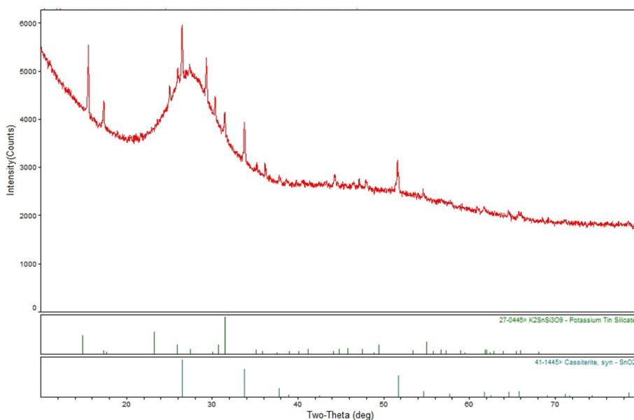
**Fig. 7** XRD spectrum of the colorless glass (shown in Fig. 6a.)
