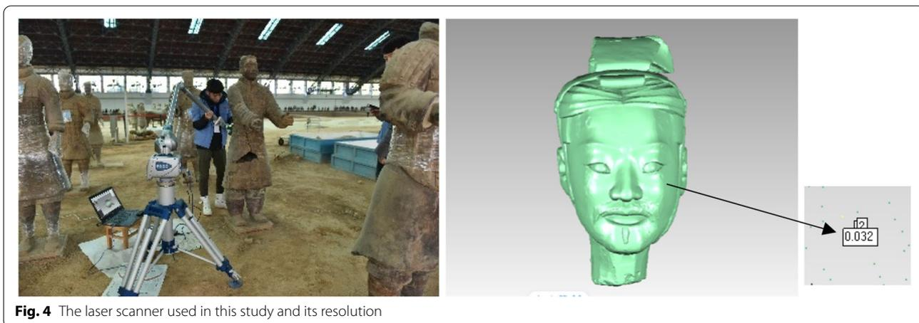
**Fig. 4** The laser scanner used in this study and its resolution
