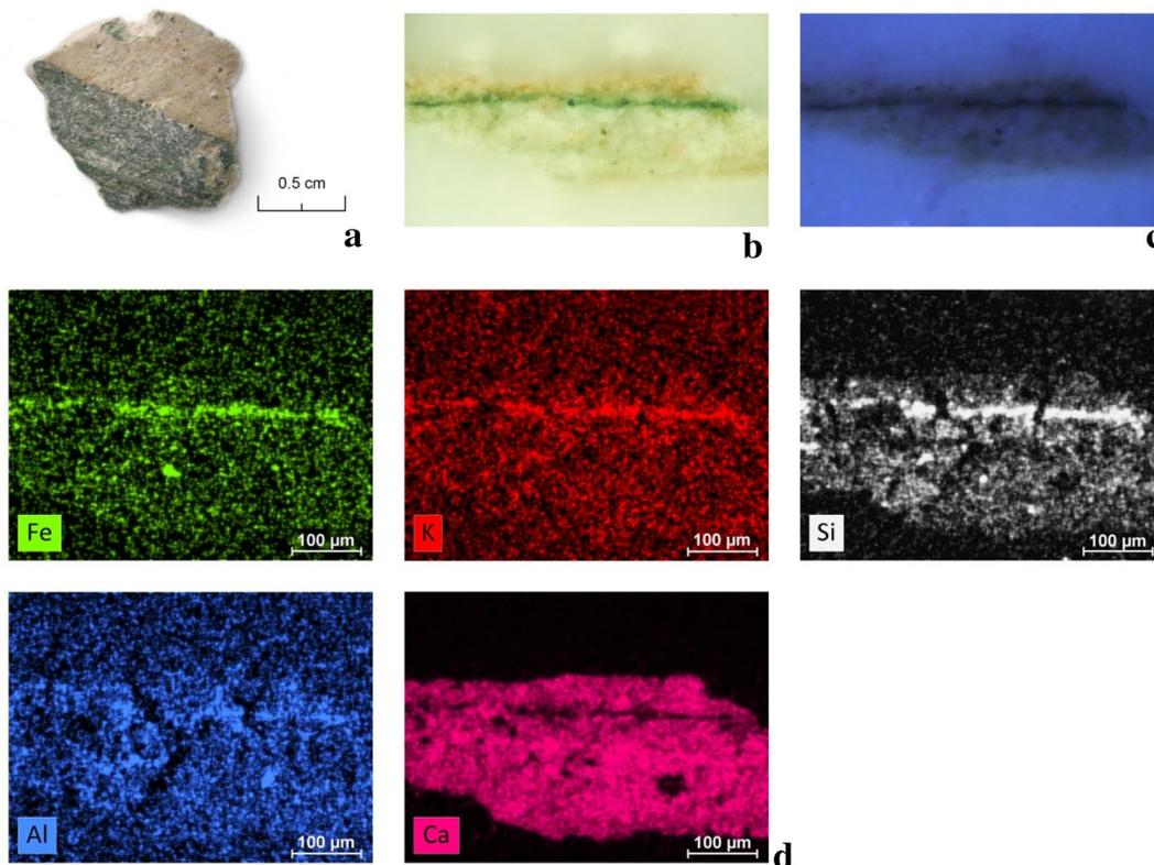
**Fig. 8** View of multicolored P4 sample (a), cross-section under visible (b) and UV (c) light, distribution maps of Fe, K, Si, Al and Ca (d)
