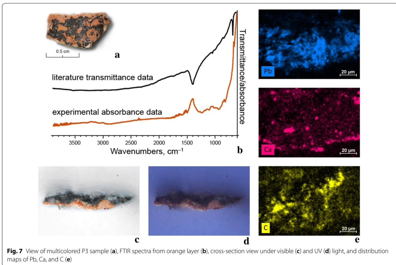
**Fig. 7** View of multicolored P3 sample (a), FTIR spectra from orange layer (b), cross-section view under visible (c) and UV (d) light, and distribution maps of Pb, Ca, and C (e)
