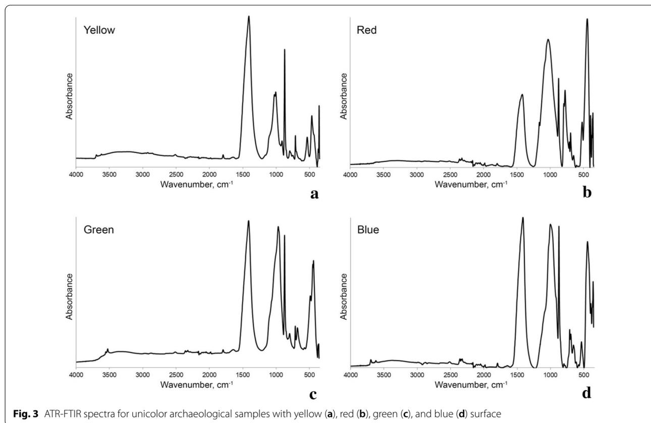
**Fig. 3** ATR-FTIR spectra for unicolor archaeological samples with yellow (a), red (b), green (c), and blue (d) surface
