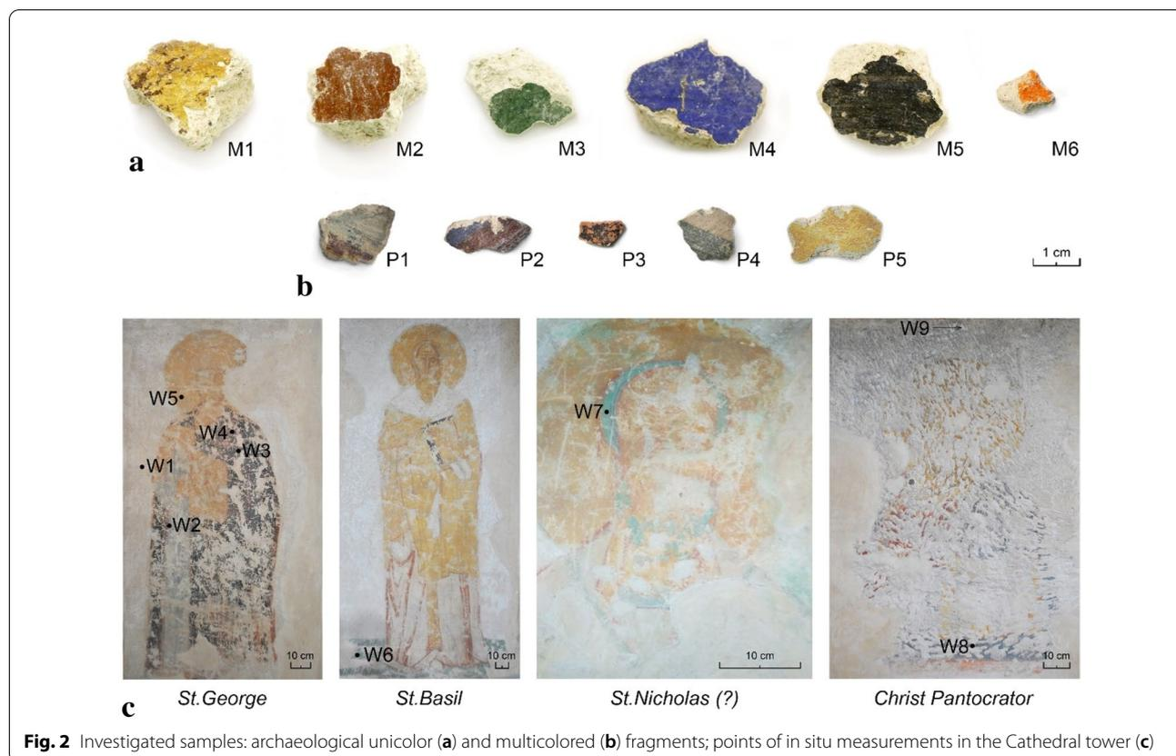
**Fig. 2** Investigated samples: archaeological unicolor (a) and multicolored (b) fragments; points of in situ measurements in the Cathedral tower (c)
