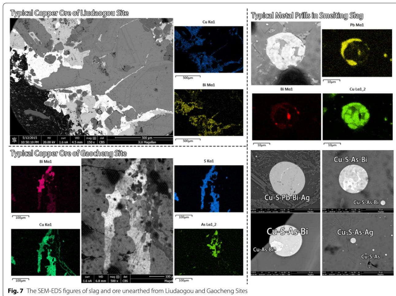
**Fig. 7** The SEM-EDS figures of slag and ore unearthed from Liudaogou and Gaocheng Sites
