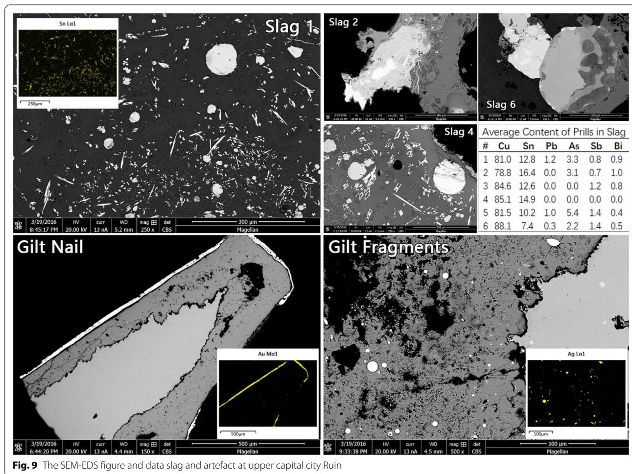
**Fig. 9** The SEM-EDS figure and data slag and artefact at upper capital city Ruin
