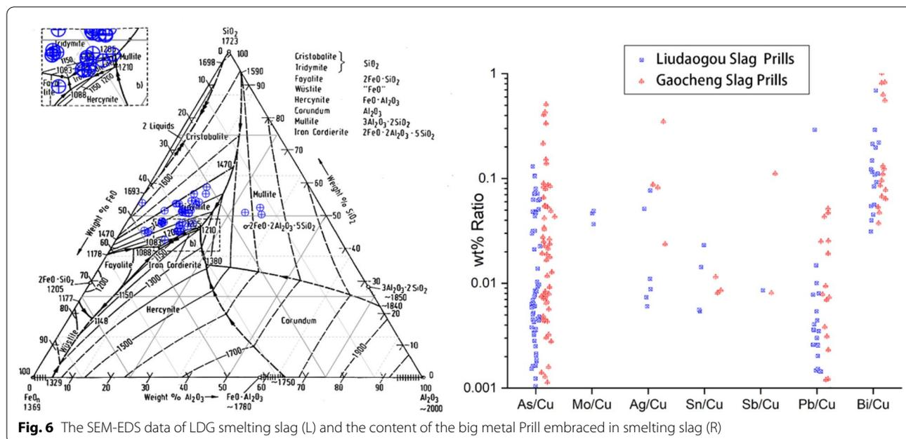
**Fig. 6** The SEM-EDS data of LDG smelting slag (L) and the content of the big metal Prill embraced in smelting slag (R)
