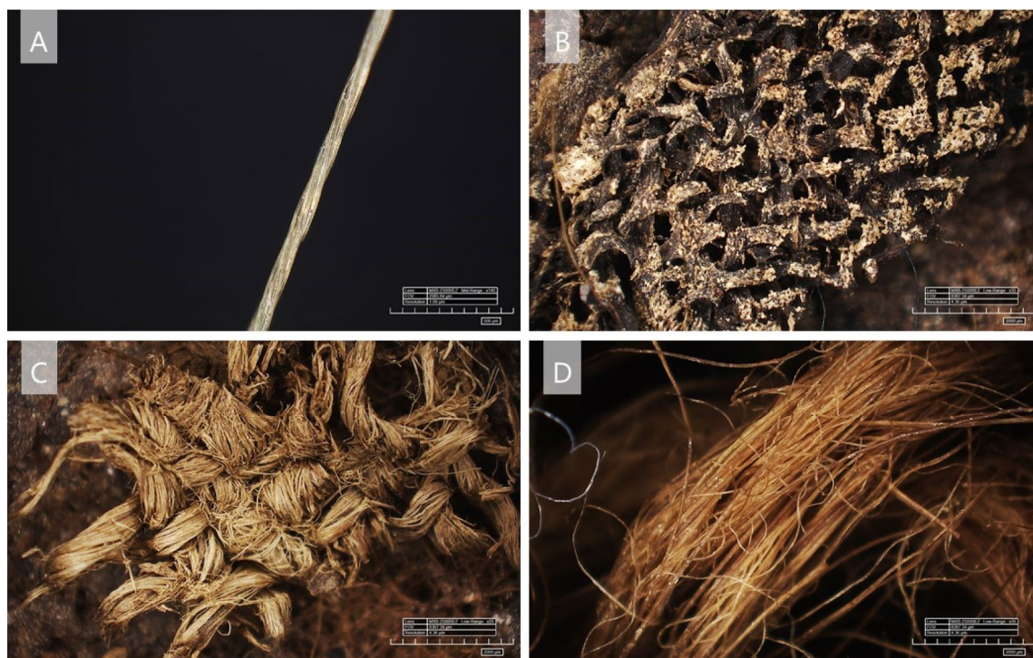
Fig. 4 Different textiles found on the breeches. A a polyester thread (Tetex, 140× magnification), B woven textile in a degraded state made of natural, likely bast, fibers (35× magnification), C a piece of woven textile, different from B with a higher density and more twist (35× magnification), D wool, which makes up the breeches themselves and the string attached to it (35× magnification)
