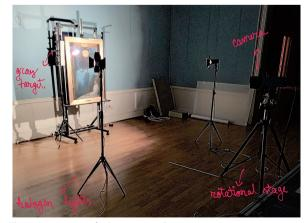
Fig. 4 In-situ setup for hyperspectral imaging
