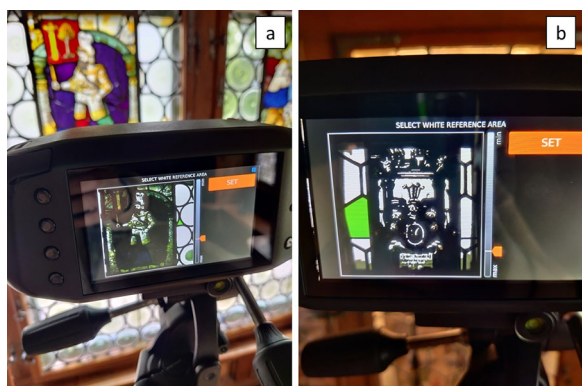
Fig. 5 Reference region selection step during the acquisition process of the case study LM-660.1 (a) and LM-789 (b). The camera shows areas with the same intensity (in white) from where the most suitable reference can be chosen (in green)
