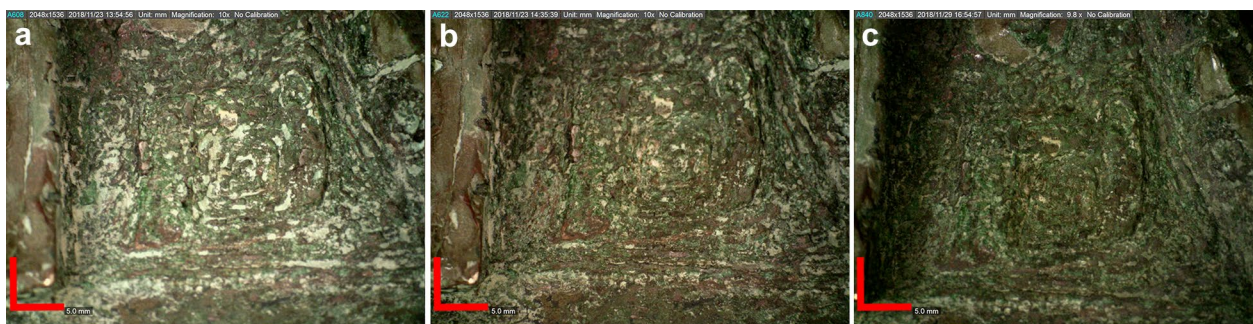
Fig. 16 Area before (a) and after laser cleaning (b) and laser-chemical cleaning (c). Scale bar: 5.0 mm
