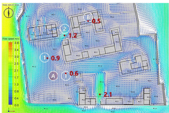
(a) Airflow before building restoration
