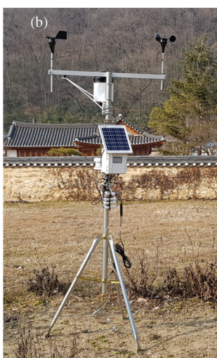
(a) Temperature and relative humidity-measuring devices (b) Wind velocity and direction-measuring devices (c) HOBOWare program (d) Flow Designer program (AKL)
