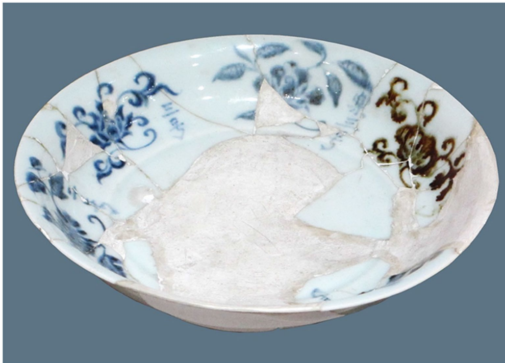
Fig. 8 Blue-and-white porcelain bowl from the Ming dynasty apparently used for the evaluation of different types or formulations of Co-based pigments (Museum of Official Kiln, Jingdezhen)
