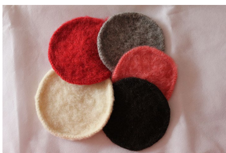
Fig. 1 Reconstructed miniature versions of the flat, circular linings inside the original early modern caps served the purpose of testing the fulling time for five different sheep’s fleece (source: Jane Malcolm-Davies)
