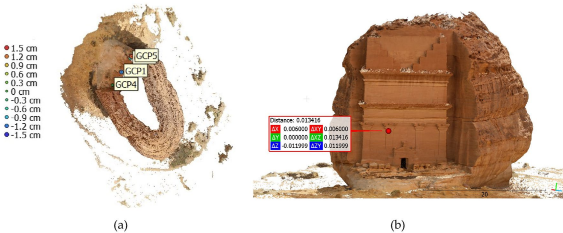
Fig. 11 a GCP estimation errors in color legend b GSD of photogrammetric point cloud
