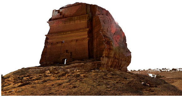
Fig. 6 The final TLS colored point cloud of the tomb
