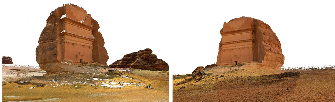
Fig. 13 Texture mapping of TLS data using independent images; the ground and surrounding areas are still textured from TLS camera
