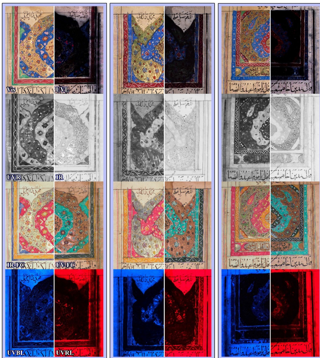
Fig. 2 Multi-band images of the gilded part of the studied manuscripts, including visible, UVL, UVR, IR, IR-FC, UV-FC, UVBL and UVRL images
