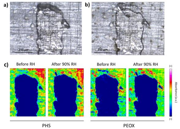
**Fig. 12** Differences between the PHS/PEOX coating on steel seen under the optical microscope. **a** Scratch of the coating before exposure to humidity in the climatic chamber and **b** Steel corrosion, after exposing the coating to 90% RH and 35 °C for 3 h. **c** Chemical distribution map of the two polymer components before and after exposure to relative humidity. The same scale in absorbance as in Fig. 10 is followed
