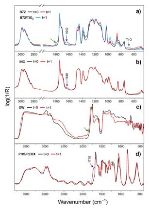
**Fig. 8** FTIR evaluation of coatings after accelerated ageing. **a** Represents B72 and TiO<sub>2</sub> spectra on steel, **b** INC spectra on steel. **c** OW spectra on brass and **d** PHS/PEOX spectra on steel. The green arrows show peak broadening, the blue arrows show new peaks and the black arrows show the characteristic peak of the Ti–O-Ti bond
