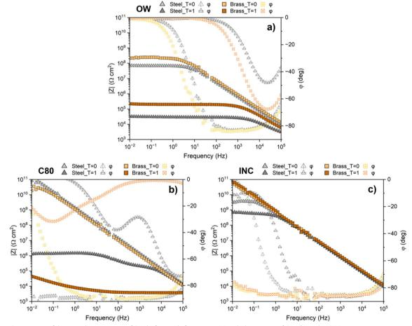
Fig. 3 Comparison of the impedance spectra of OW before and after ageing (a) with the spectra of C80 (b) and INC (c)
