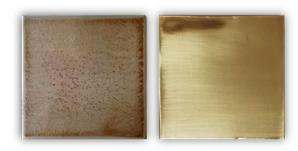
Fig. 10 Macro-photos of PHS/PEOX + CaCl<sub>2</sub> on steel (left) and on brass (right) after 48 h of drying. Corrosion is observed to be higher in the areas where more coating accumulated after application
