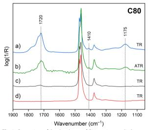
Fig. 9 Comparison of the absorbance of C80 coatings applied on steel (a) and brass (b, c) after ageing. A spectrum on steel at t=0 is added as a reference (d)
