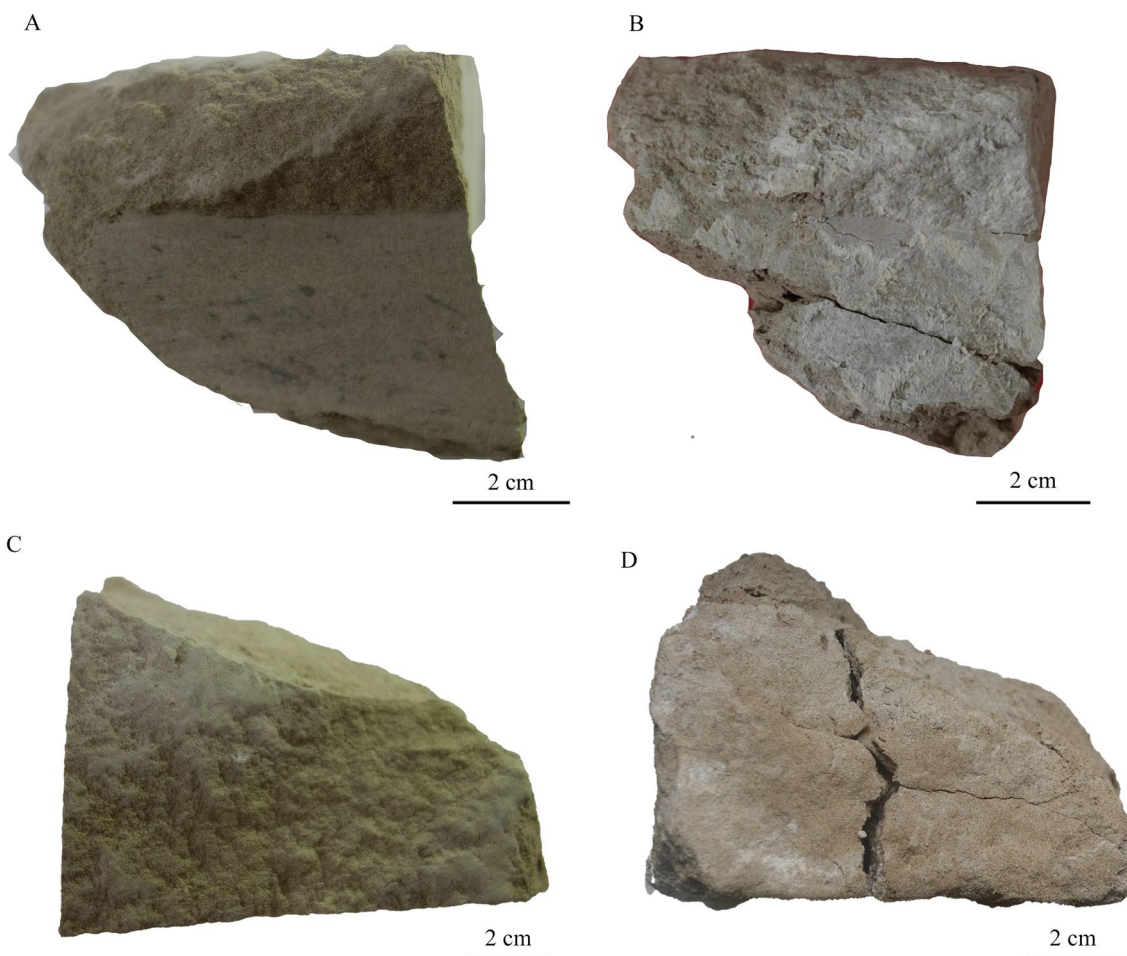
Fig. 9 The contrast between initial and desalinated rocks used the DC method. A Initial surrounding rocks. B Desalinated rock using paper pulp, C Initial surrounding rocks. D Desalinated rock using CKS121
