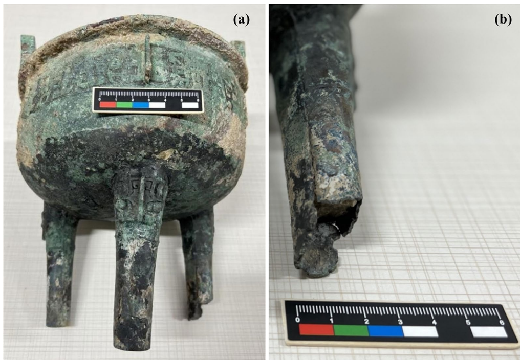
Fig. 10 Legs with clay cores and casting defects of M9:14 tripod unearthed from Zhuangli foundry in Zhouyuan, referred to Western Zhou Dynasty period. a Full picture of tripod M9:14, b leg of tripod M9:14
