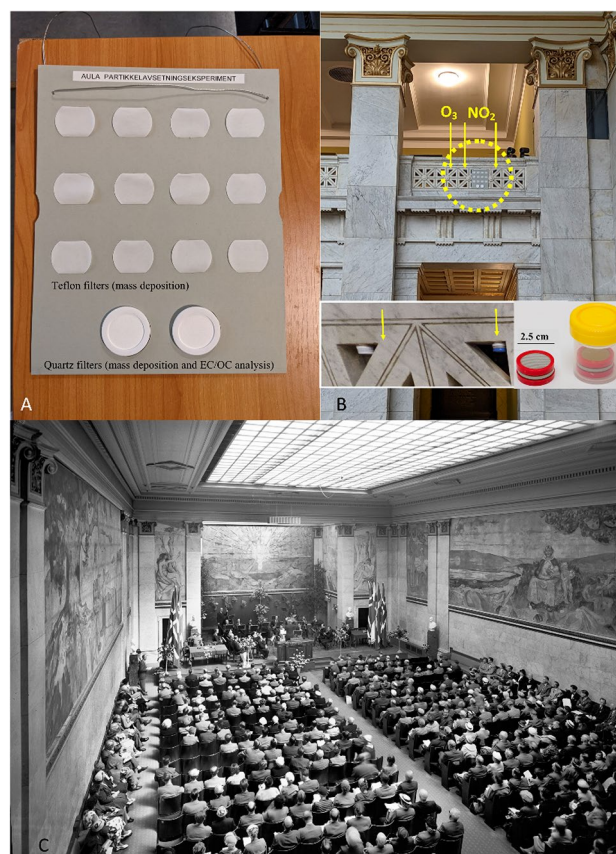
Fig. 1 The mounting of Teflon membrane and quartz filters on the cardboard plate (A), the vertical exposure of the filters, and exposure of the passive gas samplers (also seen in the enlargement) under the Aula gallery balustrade (B), and the view towards the paintings in the Aula from the gallery (C) in 1955, when grid-like thermal soiling deposits over the stretchers of the paintings on the left and right could be observed. The present room arrangement of the Aula is close to that in the photograph. C reproduced with permission from the UiO Universitetshistorisk fotobase
