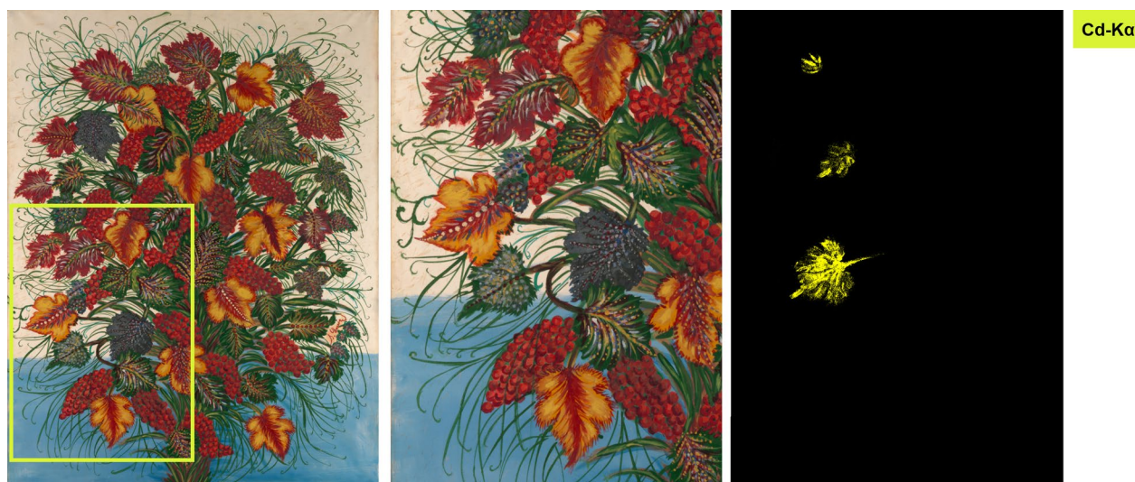
Fig. 10 (Left) Grapes with a yellow rectangle indicating the (center) detail area where (right) the elemental distribution map for cadmium (Cd-K \alpha ) was acquired by XRF scanning. The map of Cd illustrates the use of cadmium yellow. Image rights for Grapes : © 2023 Artists Rights Society (ARS), New York. All reproductions of the work(s) are excluded from the CC-BY License
