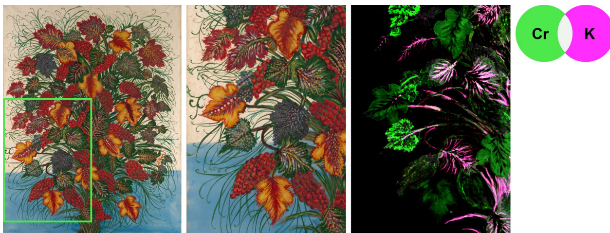
Fig. 11 (Left) Grapes with a green rectangle indicating the (center) detail area where (right) the elemental distribution maps for chromium (Cr-K \alpha ) and potassium (K-K \alpha ) were acquired by XRF scanning. The combined map illustrates the use of zinc yellow, where the co-localization of Cr and K appears near-white. The zinc (Zn) map is not shown here for clarity and can be found in Additional file 1: Fig. S2. Image rights for Grapes : © 2023 Artists Rights Society (ARS), New York. All reproductions of the work(s) are excluded from the CC-BY License
