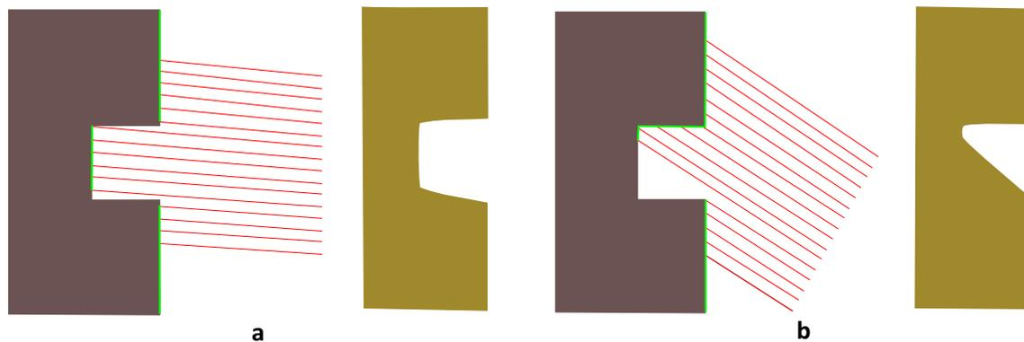
**Fig. 16** A probable reconstruction of the column carving when the laser beam (red lines) enters the carving at: **a** flat angle, **b** acute angle (On the left side of Fig. a and b there are scanned objects, and on the right side—reconstructed objects. The green lines mark the column surface visible for the scanner)
