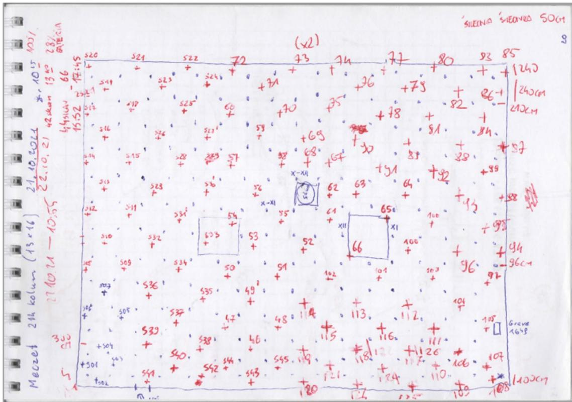
**Fig. 9** The appearance of the handwritten scanning plan (blue dots represent columns and red crosses—scanning positions) and its implementation (red numbers with possible repetitions)
