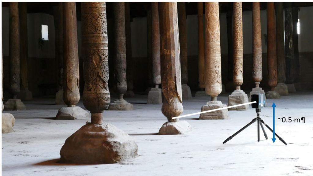
**Fig. 7** Height of the scanner above the floor level ensuring correct scans
