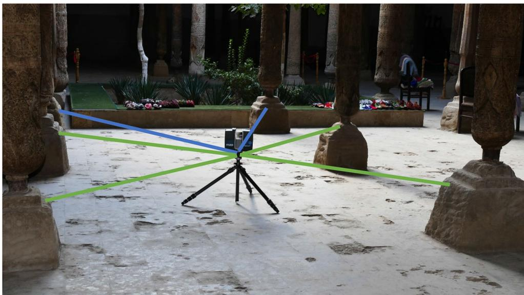
**Fig. 10** Scanning the interior of the mosque from the centre of the square between the columns. Indicated are columns in the near range (green) and far range (blue) for this scanner position
