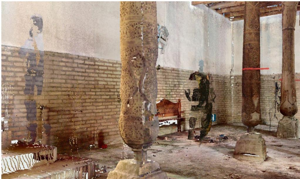
**Fig. 12** An example of interference in the acquired scans
