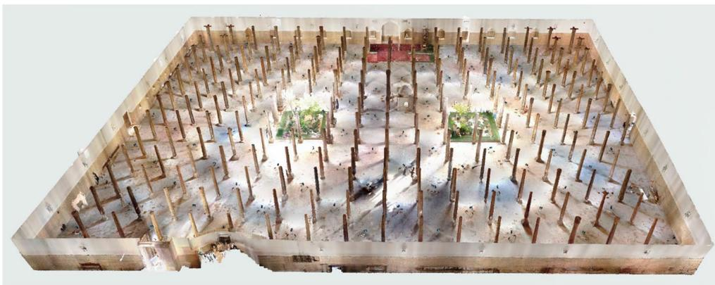
**Fig. 11** An overview of the combined point cloud from the Juma Mosque scanning with scanning positions (marked with a blue scanner hardware shape between the columns). Some of them are duplicates
