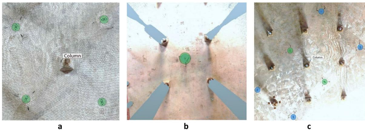
**Fig. 8** Scanner placement positions: **a** four scans per column, **b** one scan simultaneously for four different columns, **c** minimum number of 6 scanner positions to obtain visibility of the entire surface of the column (Column) (green—close position and blue—further position markings are scanner placements)
