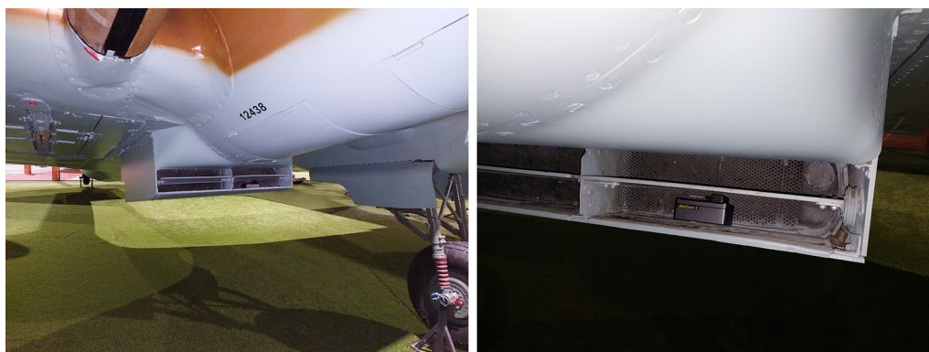
Fig. 2 Logger AirCorr I placement in the monitored hangar within aircraft Ilyushin IL-2m3 Shturmovik. Overall view (left). Detail on aircraft intake (right)
