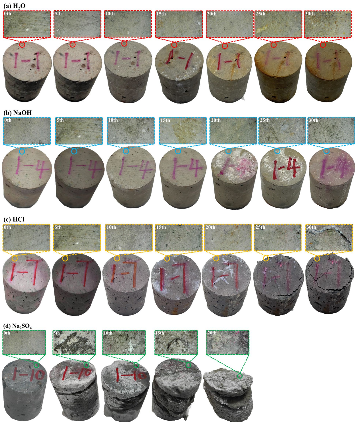
Fig. 14 Appearances and micrographs of samples after different cycles
