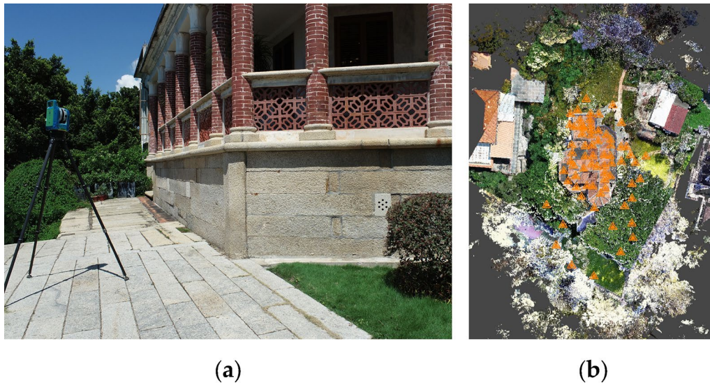
Fig. 7 a Trimble X7 laser scanner scanning the building; b The distribution of TLS survey sites
