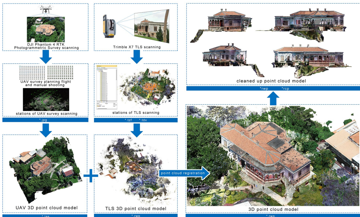
Fig. 10 The workflow of point clouds registration
