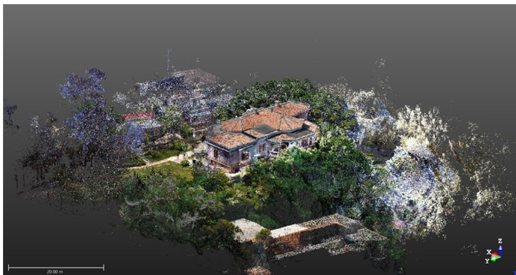
Fig. 11 The result of point clouds registration
