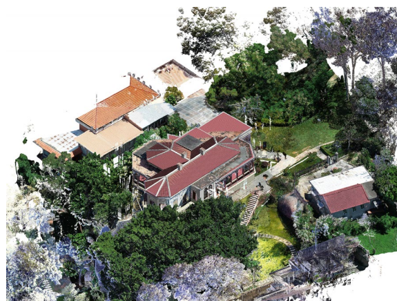
Fig. 19 The result of importing point clouds into HBIM, as a support for modelling or a supplement to HBIM
