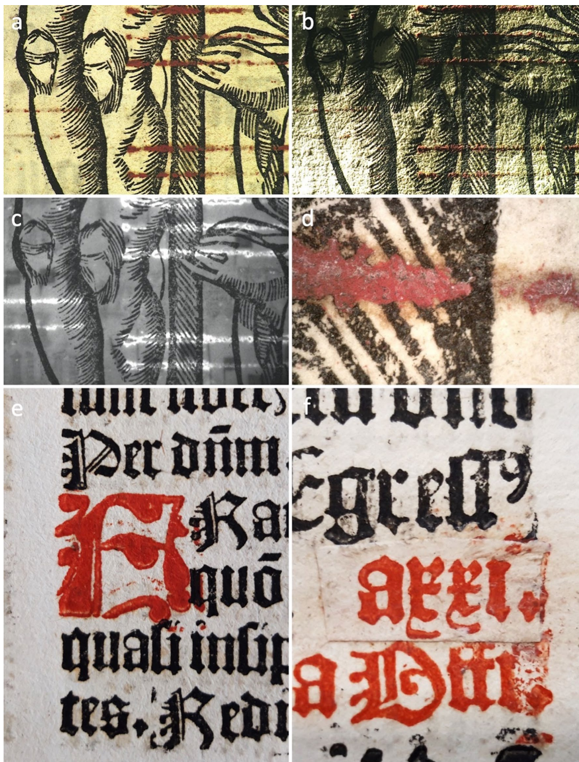
Fig. 6 a–c Migration of red ink through the paper in VIS (a), raking light (b) and infrared fluorescence (c). d Detail of the agglomeration of the red ink. e Magnified image of the printed text, showing that the printing sequence was first red, then black. f An error in printing has been corrected with a slip of paper
