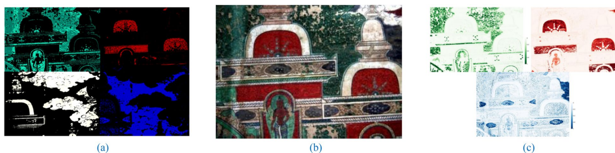
Fig. 4 Segmented recognition results of single pigment spectrum considering ion absorption: a spatial distribution of four typical pigment homogeneous regions; b true color image; c improved K–M model and sparse demixing results (abundance maps of unmixed lithic green, cinnabar and lapis lazuli)
