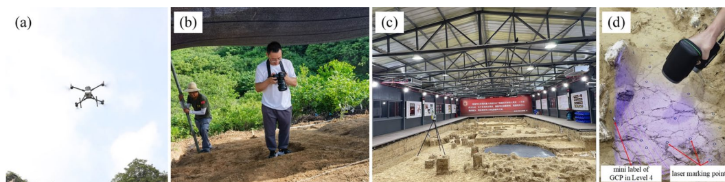
Fig. 4 Data collection methods. a Data collection through aerial photogrammetry. b Data collection through close-range photogrammetry. c Data collection through terrestrial laser scanning. d Data collection through portable laser scanning
