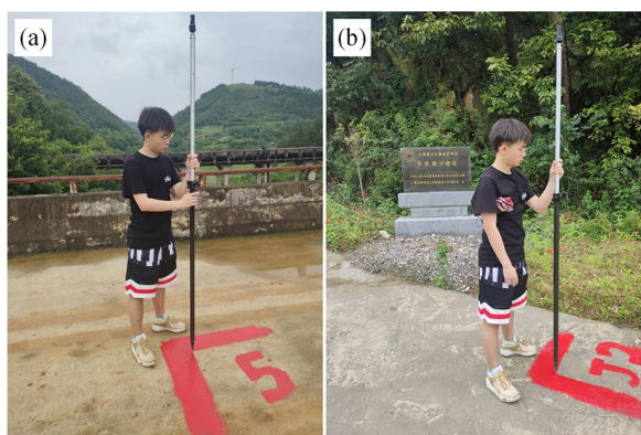
Fig. 6 The appearance of GCPs at Level 1. a, b Show two different GCPs at Level 1 and scenarios using RTK to survey their geographic coordinates
