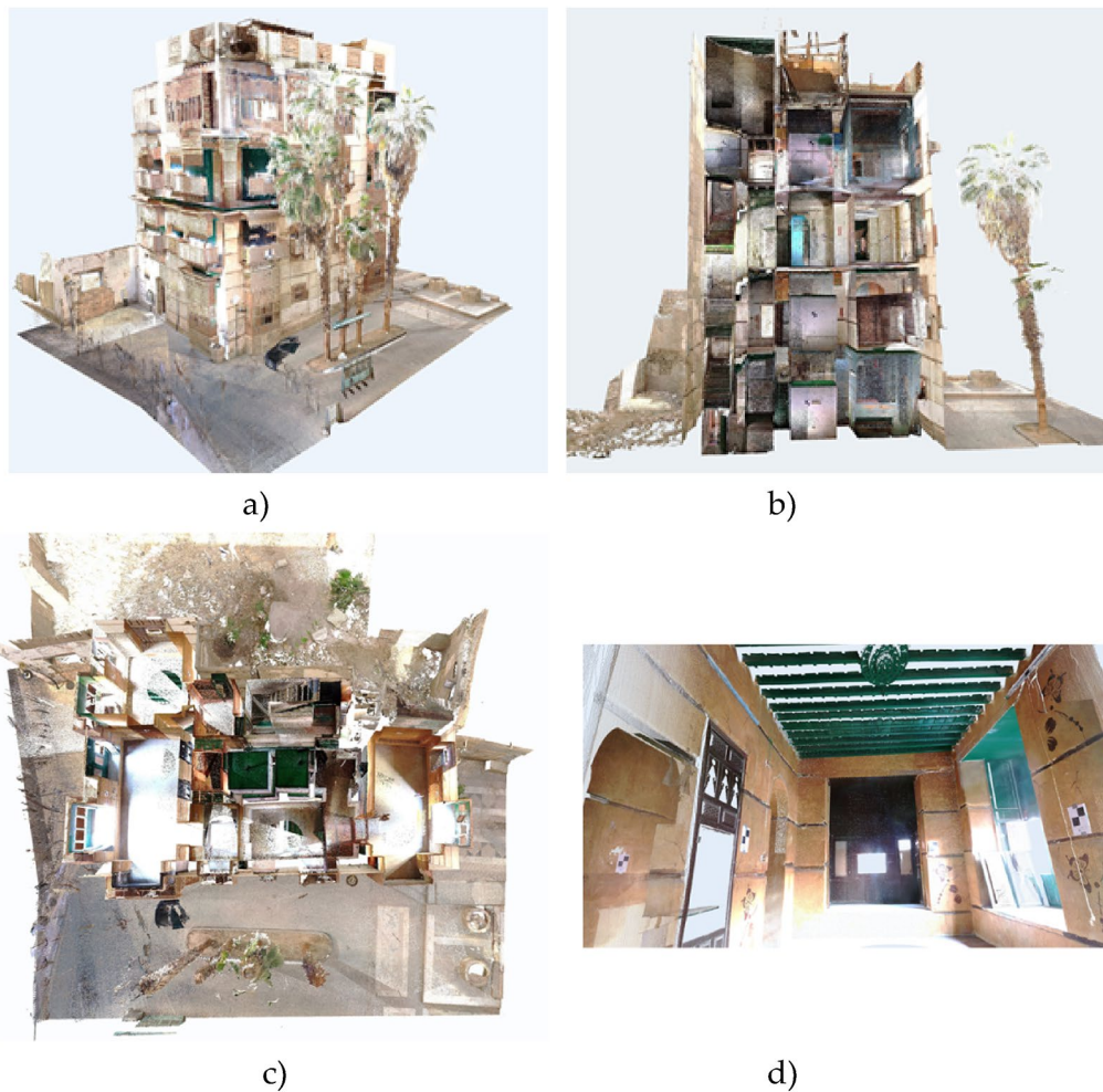
Fig. 8 a The final model of the building b long section c Cross section d Interior scanning
