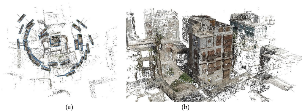
Fig. 10 UAV a camera position and the initial tie points b point cloud densification
