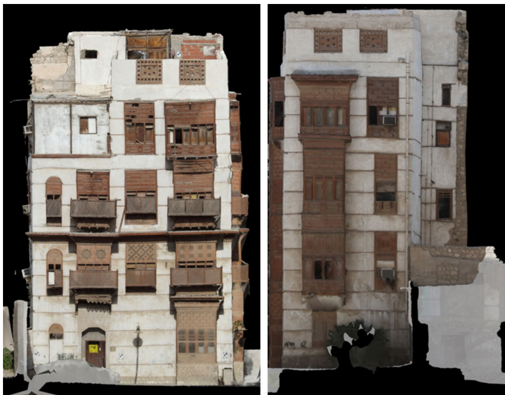
Fig. 14 True orthophoto using UAV photogrammetry
