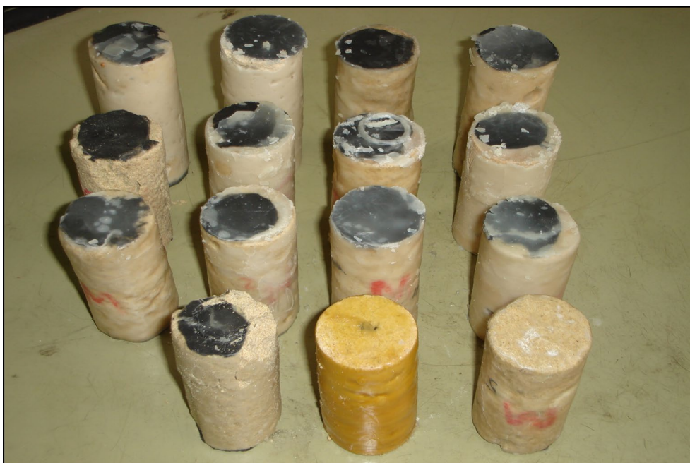
Fig. 3 Part of the cylindrical rock specimens, who have been used in Triaxial Compression test
