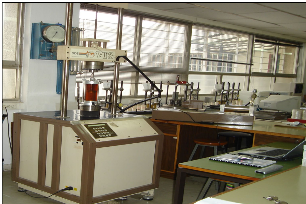
Fig. 4 Triaxial compression test equipment. The cylindrical specimen placed inside GDS cell is loaded vertically using the compression machine. (GDS instruments limited, England)
