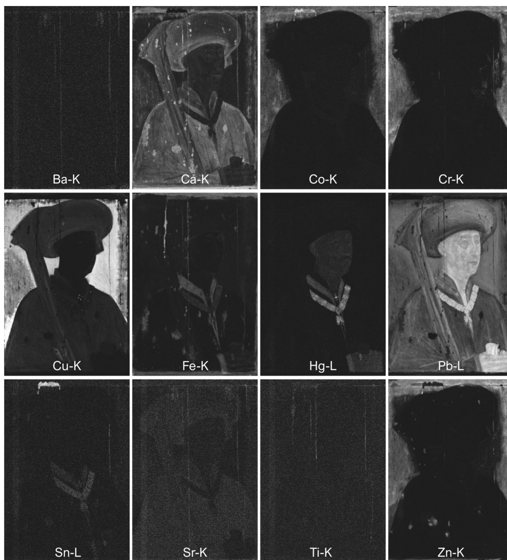
Fig. 7 MA-XRF scans of the Portrait of Philip the Good (Dijon, Musée des Beaux-Arts). The original images are adjusted for brightness and contrast to improve the readability of the image
