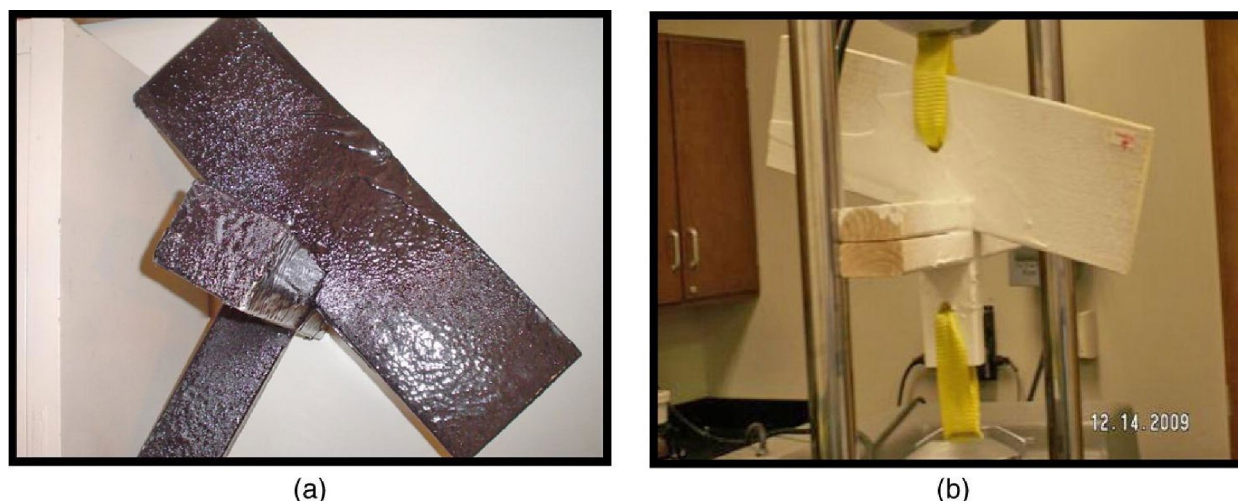
Fig. 22 Schematic diagram of polyurea coating reinforcement [135] (a) Black polyurea material with high elongation and low elastic modulus (b) White polyurea material with low elongation and high elastic modulus
