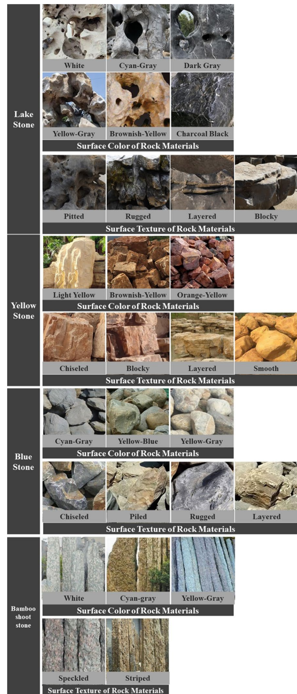
Fig. 1 Classification and characteristics of rock materials
