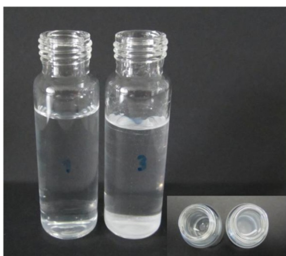
Figure 6 Stability of calcium hydrogen carbonate in solution. Calcium hydrogen carbonate in pure water (left vial) and in mixture of water and ethanol (2:1) (right vial) after exposure at ambient conditions for 3 hours. Precipitation of the calcium carbonate at the bottom of the vial is clearly visible in the mixture.
