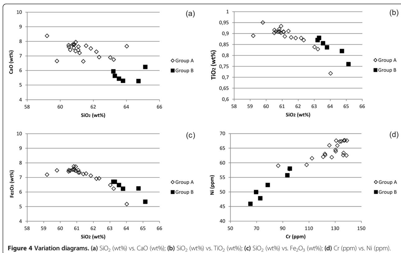
**Figure 4** Variation diagrams. (a) SiO<sub>2</sub> (wt%) vs. CaO (wt%); (b) SiO<sub>2</sub> (wt%) vs. TiO<sub>2</sub> (wt%); (c) SiO<sub>2</sub> (wt%) vs. Fe<sub>2</sub>O<sub>3</sub> (wt%); (d) Cr (ppm) vs. Ni (ppm).
