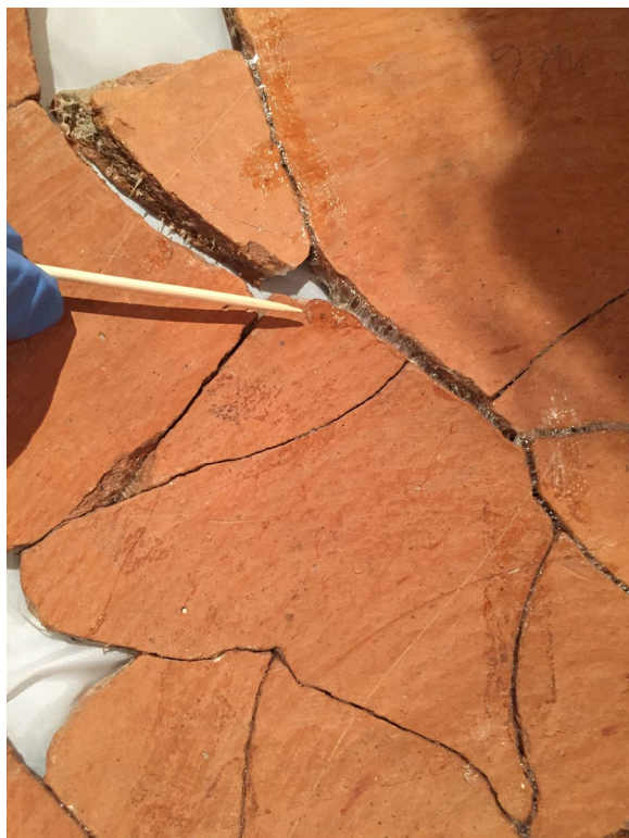
Fig. 2 Example of adhesive failure, s1342, identified via FTIR-ATR spectroscopy as containing primarily PVAc + CN as a secondary polymer. Vessel 1970.0478, Palestine, Jerusalem Cave 1, The University of Melbourne Middle Eastern collection. Photograph: Emily Noake
