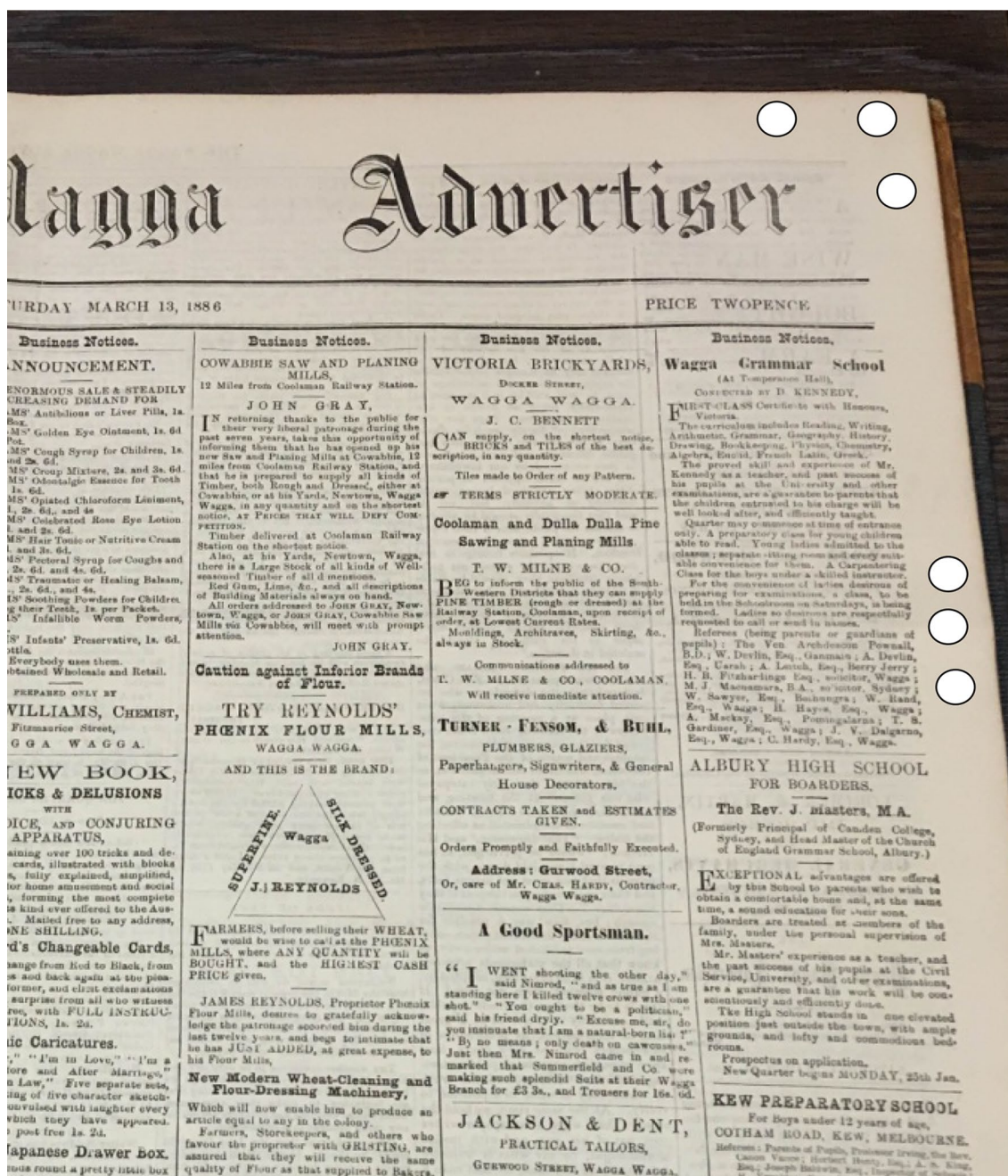
Fig. 2 Copy of the Wagga Wagga Daily Advertiser from 1886. The figure shows six white circles indicating the typical positions used to make two sets of triplicate measurements on a page close to the beginning and centre of each folder. Such sites were used for the X-Rite I1 Pro, with triplicate measurements made for the mid page section in fewer selected journals using the iPhone6S
