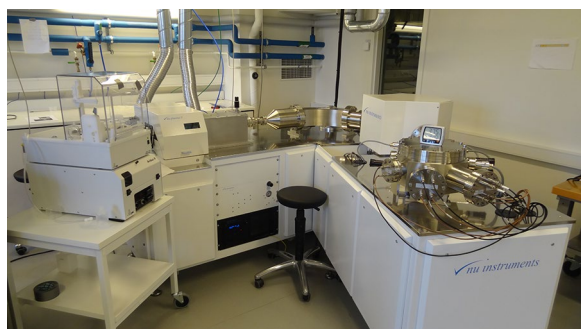
Fig. 2 An MC-ICP-MS spectrometer (Nu Plasma II) at the Department of Geological Sciences, Swedish Museum of Natural History, Stockholm. Photo: Melanie Schmitt
