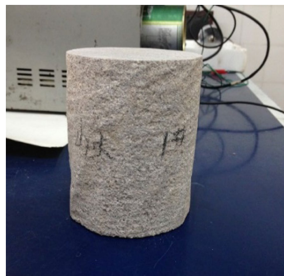
Fig. 1 The processed rock specimens (both diameter and length are 10 cm)
