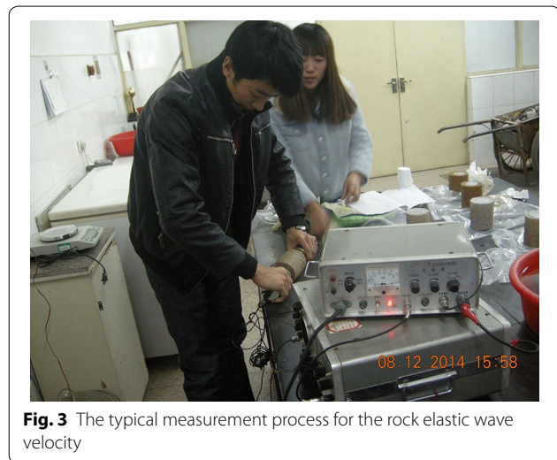
Fig. 2 Rock elastic wave velocity measurement process
