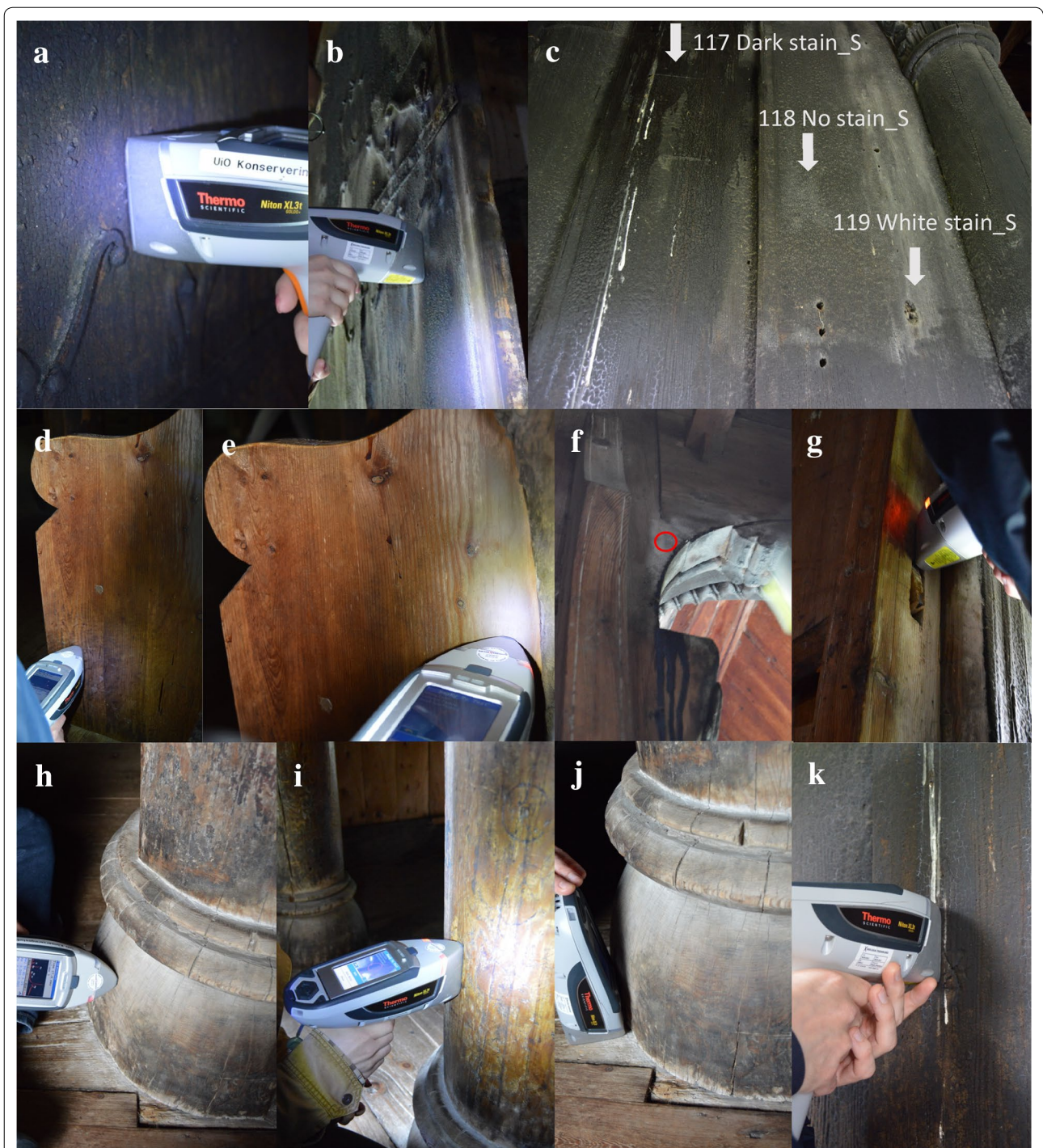
Fig. 5 Locations of the XRF measurements. a Measurement 111 with no white substance and b measurement 113 with white substance were taken on the southern exterior door. c Measurements 117, 118 and 119 (marked with white arrows) on the exterior wall left of the southern entrance with staining. d Measurement 110 with no white substance and e measurement 106 with white substance were taken on the bench inside the church. f Measurement 125 was taken on the white substance on the wall by the entrance (marked with a red circle). g Measurement 126 was taken on the white substance on the crossbar. h Measurement 120 was taken on the stave base with a white substance. i Measurement 122 was taken on the stave without a white substance and j Measurement 121 was taken on the floor with a white substance. k Measurement 116 was taken on the bird droppings
