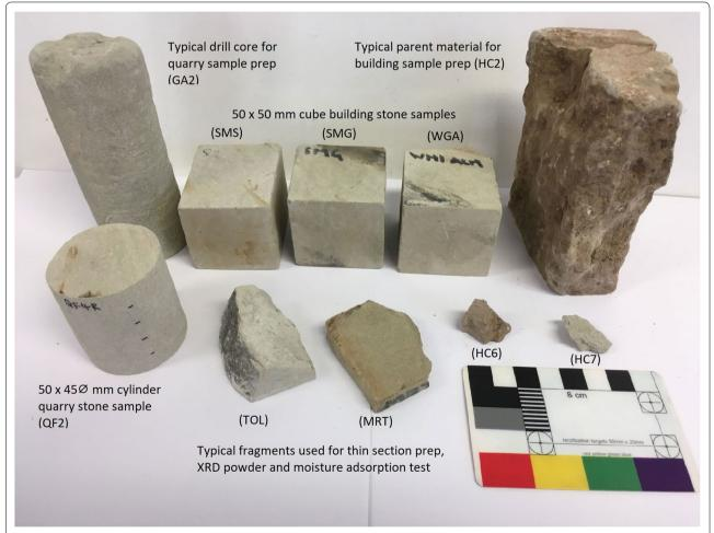
**Fig. 4** Selection of Reigate Stone specimens showing variation in colour and texture across different samples used in this study and explaining different sample dimensions
