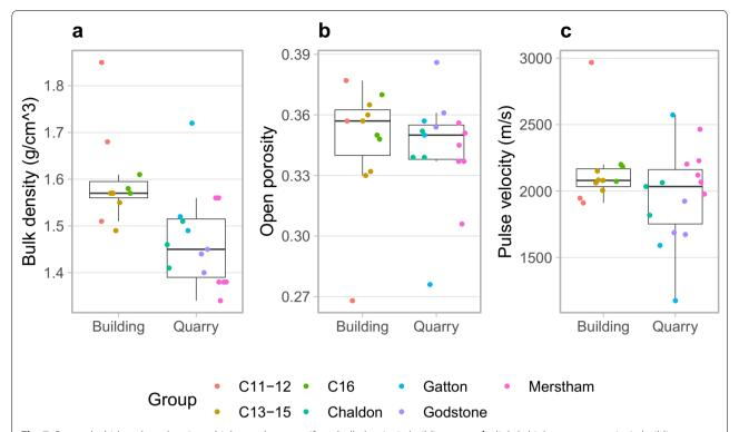
**Fig. 7** Box and whisker plots, showing **a** higher and more uniform bulk density in building stone, **b** slightly higher open porosity in building stone, and **c** more uniform response to pulse velocity measurement in building stone. Central line of box depicts mean value; lower and upper edges of box correspond to 25th and 75th percentile (IQR); whiskers extend to the largest/smallest value within 1.5 \* IQR
