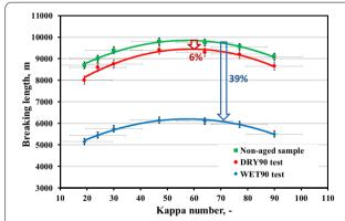
**Fig. 2** Effect of paper-ageing conditions on changes in the breaking length of papers with different lignin contents
