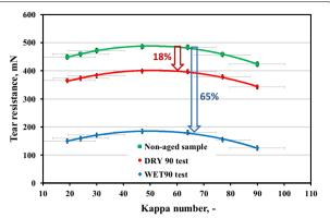
**Fig. 3** Effect of paper-ageing conditions on changes in the tear resistance of papers with different liquin contents
