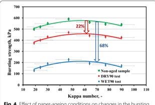
**Fig. 4** Effect of paper-ageing conditions on changes in the bursting strength of papers with different lignin contents
