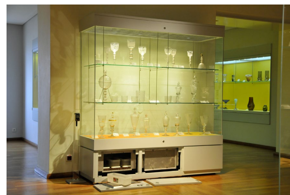
Fig. 1 Display case for ‘sick’ glass at Veste Coburg using magnesium chloride solution in plastic containers in the lower part during maintenance. © H. Grieb
