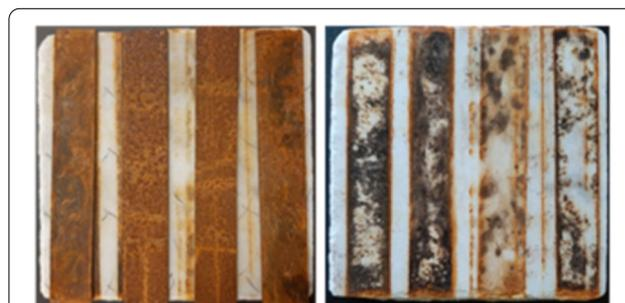
**Fig. 1** On the left, sample C of Carrara marble with superimposed iron bars; on the right, the stains produced
